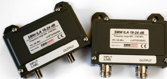
The Line Amplifiers are equalized to compensate the cable attenuation and other losses. Comes either with F-, N- or SMA-connectors. DC bypass is standard. Options include Separate DC power input via connector (F, N or SMA) or via two thin cables, 10 MHz bypass and high currency 5 A bypass.
