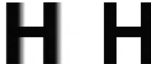
Using a Philips screwdriver, adjust the EQ control until any shadowing effect, as illustrated on the left hand side, is reduced to an acceptable level, as on the right. Adjust the GAIN control until you achieve a satisfactorily bright picture.
