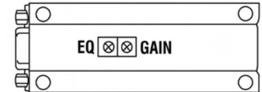
A good method to check and adjust the picture quality is to display a high contrast image, with vertical edges, on the remote screen. Launch a word processor and type a large capital 'H' in the centre of the screen. Use a bold black font, with a size of 72 points or higher, on a white background.
